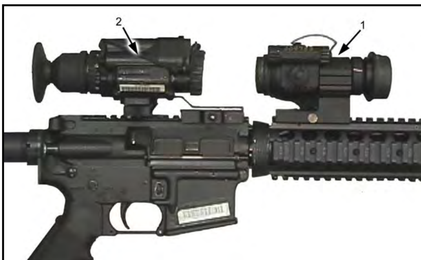
Figure 2-26. Mounting the M68/AN/PVS-14 combination on an MWS.
