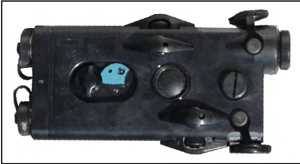
Figure 2-30. AN/PEQ-2A target pointer illuminator/aiming light.
