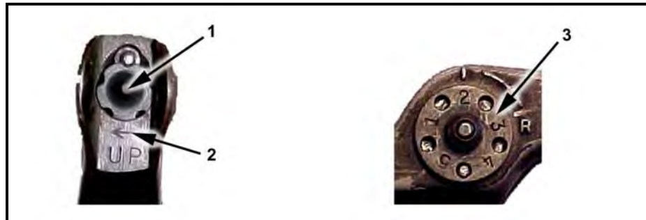
Figure 2-2. M16A1 rifle mechanical zero.
