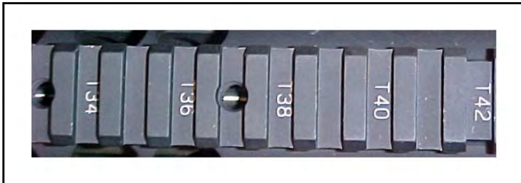
Figure 2-16. Address markings on RAS.
